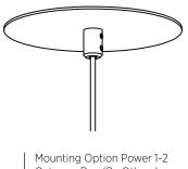
Mounting Option Power 1-2 Octagon Box (By Others) Installed in drywall, wood or concrete ceiling
