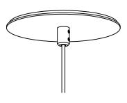
Mounting Option Power 2-2 65mm Diameter Box (By Others) Installed in drywall, wood or concrete ceiling
